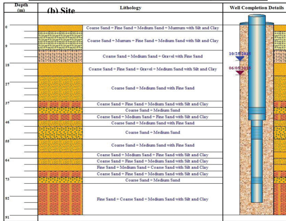
FIGURE 20.3 Well logs and well completion details at: (a) site PHTC and (b) site PFDC (Kharagpur, India).
