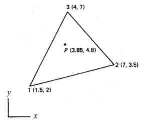
[10M] MT 0422\_A\_23 9. For the plane stress element shown in figure, evaluate the stiffness matrix . Assume the modulus of elasticity  $E = 210 \times 10^{3} N / mm^{2}$ , Poisson's ratio  $\mu = 0.25$  and element thickness t = 10mm. The coordinates are given in millimeters.
